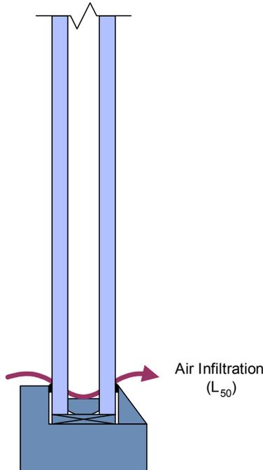
Air leakage occurs primarily through joints in the window frame, poorly sealed gaps between opening lights and outer frames and to a much lesser extent through gaps between the glass and the surrounding frame.
