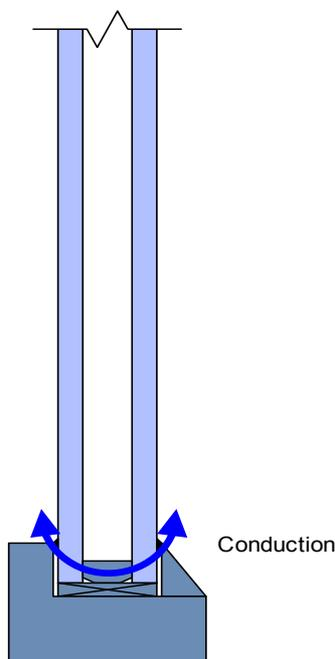
The effort of getting the  $U_{\text{frame}}$  down to the legislative requirements of the Building Regulations is often concentrated on the frame and the low-E coating. This can result in the use of expensive coating technology when a similar result can be more easily achieved at a lower cost by using new 'warm-edge' technology in sealed unit construction. The benefit of using warm-edge spacers is dramatically shown in
