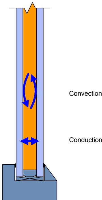
Gas filling replaces the air or nitrogen with an inert gas such as argon or krypton. These gases are more viscous and slower moving than air or nitrogen and minimise both the convection currents and the conduction of heat through the glazing gap.
