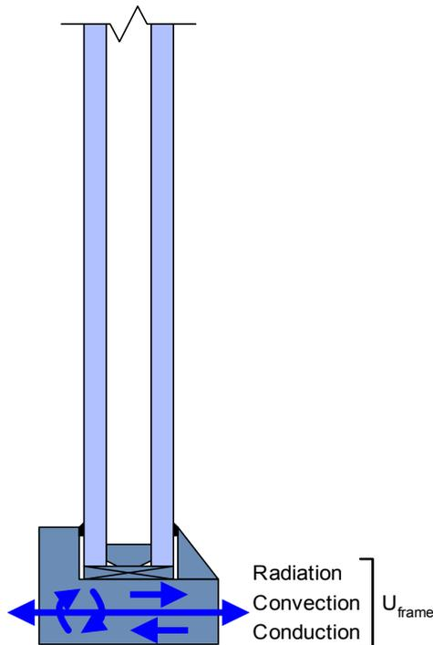
Minimising the  $U_{\text{frame}}$  is a key objective for profile designers in any material. There is potential for improvements in all current frame systems and materials but Building Regulations and current standards for safety, durability, security and wind loading make it unlikely that these improvements will be greater than 0.1 to 0.2 of  $U_{\text{frame}}$ . This will therefore have a proportionately less impact on the whole-window U value ( $U_{\text{window}}$ ).
